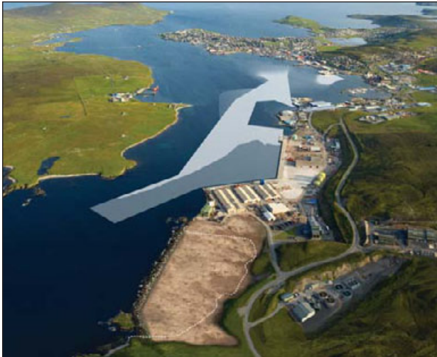
Lightest areas in photomontage above are dredged to 9 metres. The reclamation area in foreground extends to 14.4 acres.
