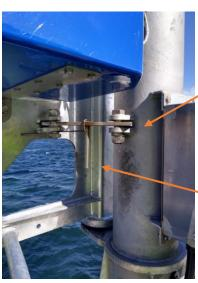
Locking mechanism in place to prevent crane swinging. Crane **MUST** be left in the "locked" position when not in use.
