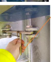
Release mechanism by pulling handle to allow crane to swing.
